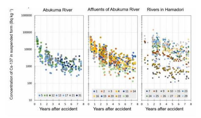
FIG. 3. Decline of <sup>137</sup>Cs in suspended matter of rivers in the Prefecture, 2011–2019 (Image: Fukushima Prefecture)
